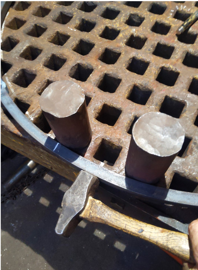
Use the hammer and a set of pins to open a bend
