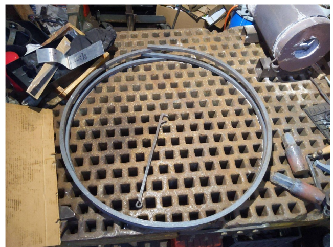
Two 37\frac{1}{4} " rings bent by hand from \frac{3}{4} " square bar. All bending was done with pins and wrenches on the acorn table
