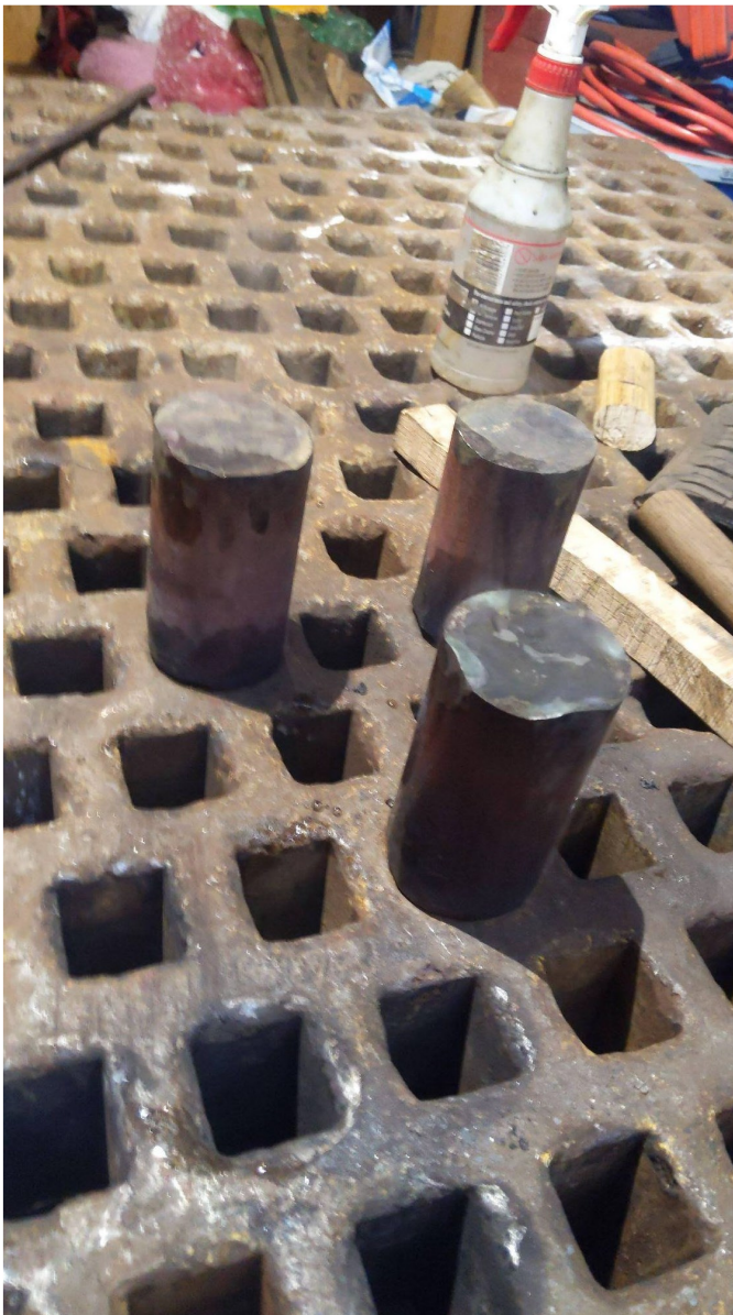
Bending pins made for an "acorn" style platen table. Forged from 2" mild steel, two pins are often enough to create a bend
