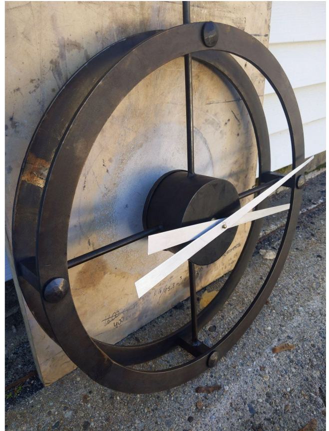
A clock with a frame made from \frac{1}{4} " x 1\frac{1}{4} " flat bar stock. Rings were bent undersize on a friend's Hossfeld bender and opened up with a hammer and pins on the acorn table
