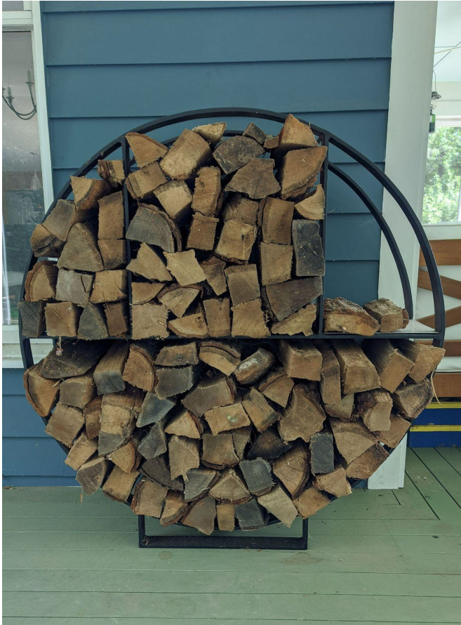
A log holder with two 36" OD rings bent "the easy way" from 1/4" x 1.5" flat stock (or something in that neighborhood, this job was a while ago). Bends were accomplished with pins on the acorn table and by using the measurement techniques detailed in points 6, 7 and 8.
