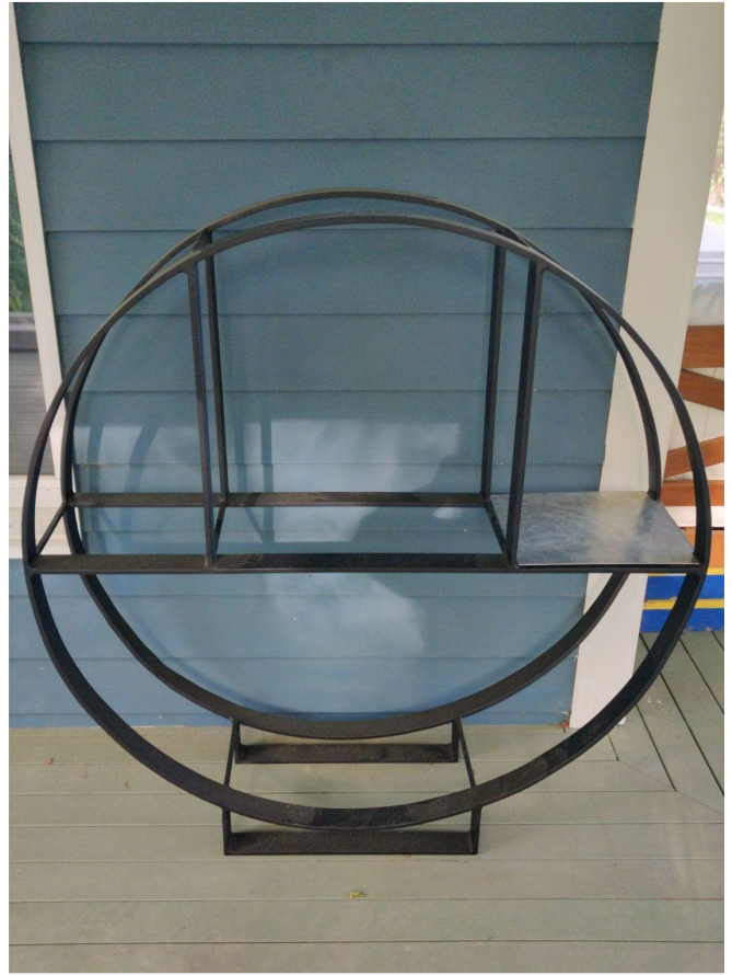
A log holder with two 36" OD rings bent "the easy way" from 1/4" x 1.5" flat stock (or something in that neighborhood, this job was a while ago). Bends were accomplished with pins on the acorn table and by using the measurement techniques detailed in points 6, 7 and 8.
