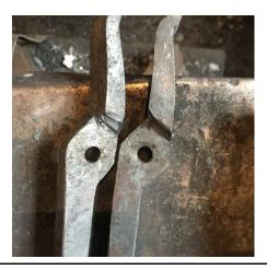
**Tip #6:** Closer to the rivet = more torque. This may be intuitive for most smiths but it bears repeating: The closer the workpiece is to the pivot point, the more gripping force the smith can apply by squeezing the reins. I have a pair of tongs I made specifically for gripping the poll of axes. By keeping the bits under an inch I am able to get a good secure grip while planishing cheeks and edges.
