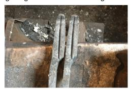
**Tip #5:** Add a notch at the transition of the bits and boss. Similar to putting a hollow in bits like we did in the last tip, a small notch at the juncture of the bit and boss creates, when the tongs are assembled, a hollow that can grab onto points or corners of the work. After all, you can't (or at least shouldn't) hit what you can't hold. I remember this tip came to me from an old issue of The Anvil's Ring but I wasn't able to find the author in my stack of back issues
