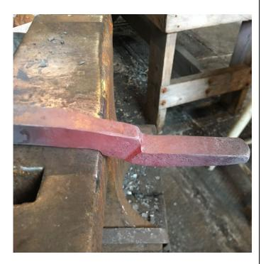
Tip #8: Make your Box-jaws more versatile. When making box-jaw tongs, make the width of the box the same as the distance from the boss to the 'wings'. This allows stock to be held in line as well as perpendicular to the tongs. On some very wide box jaw tongs this is impractical, so it's a guideline, not a hard and fast rule.
