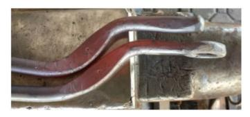
10. Punch and drift the pivot hole. I punch to slightly under 3/8", then drill out to 3/8". A 3/8" rivet fits nicely.
