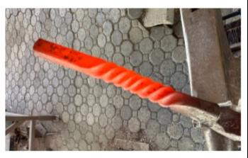
As with the test pieces Will drew the sections down to 3/8" thick, then punched & drifted.
