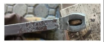
Then he drifted over both a bolster plate and on the anvil horn.
