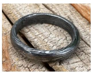
Will didn't have the green polishing compound up until this point, so he polished the ring once more at this step with just the green compound. Last step was to seal the ring with protectaclear. It's not permanent but by the time it wears off we're hoping oils from the skin will prevent oxidation.
