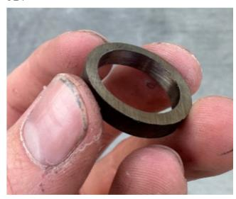
A forstner bit was used on a drill press to make a perpendicular hole for the roughed ring to seat itself in, then a right angle guard to guide the ring against the grinder to make each side of the ring parallel and to get the width of the ring where it needed to be.
