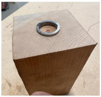
The "final" ring thickness was then ground manually by rolling on a surface to see which sides had more mass to grind down. Layout fluid and calipers could have been used also.
