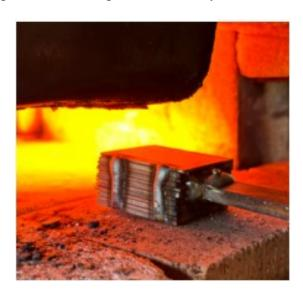
We brought the (propane) forge up to welding heat, then the first job was to set the weld. Fluxed, then forge welded.
