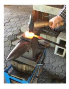
Will then alternated between drawing dies in the hydraulic press and the hand hammer, to draw the billet out to 5/8" x 5/8".
