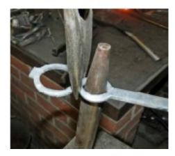
Again, round up the hole on the anvil's horn, or a cone mandrel.
