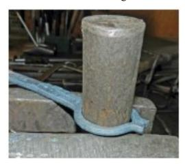
Round up the hole on the anvil's horn, or a cone mandrel. Taking as many heats as necessary.
