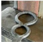
Grind off the end tab so the bottom circle visually has a consistent wall thickness, then break those corners too.
