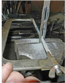
Remove most of the chisel "rag" with the saw, and cut to the ends of each slit.
