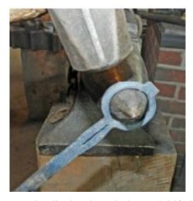
Open the slit, then heat the bar and drift the second hole. Tweak the area between the two holes so they are aligned above each other.
