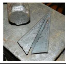
Heating the ornament makes deeper impressions. Heat the tree and create the impression of boughs with a straight peened hammer on the front of the tree. Then decorate the tree by adding ornament impressions with a round eye punch, chiseling in garland swags, stars or twinkling candles. Wire brush clean, then highlight with a brass wire brush as it cools. Lastly, drill a small hole at the top for a wire ornament hook. Add a bead if you like.
