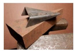
Progressively hammer the sides down onto the back of the tree, using a wide flat chisel and the anvil's step to work against. Work the material to have a smooth transition at the point.
