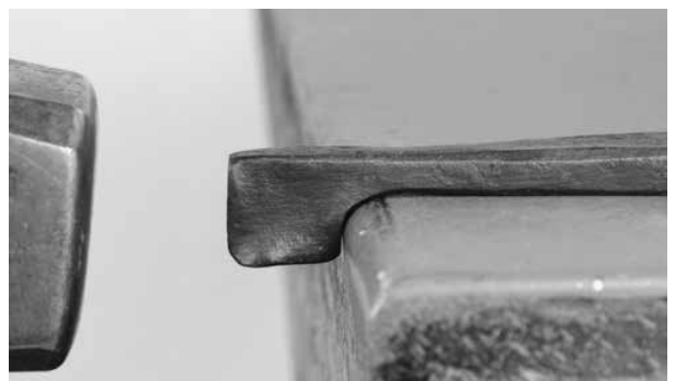
Upset the flag to form a square of material, holding your hammer vertically as you work
