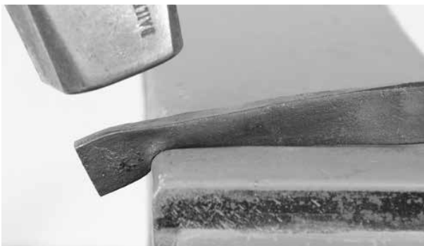
Shoulder in half the width of the bar. That should leave you with a \frac{3}{8} " square neck
