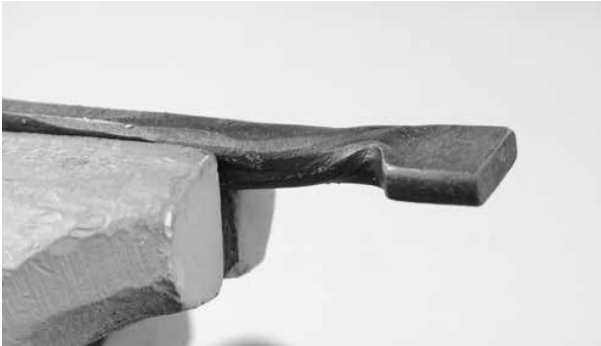
Twist at the vise using a pair of scrolling tongs
