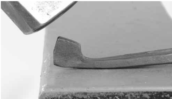
Angle your hammer as you pull in what was the lower corner. Drop the hammer angle as you work
