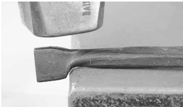
Return to the soft, offside edge and re-establish your taper to the parent bar
