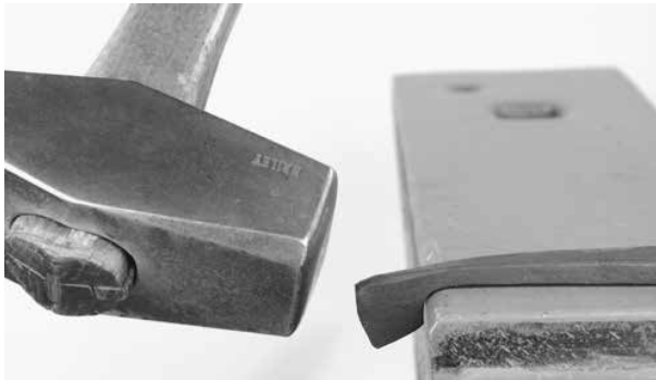
The last move will have made the lower corner of the flag stand out
