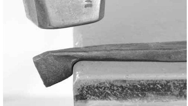
I like to bring the tip of the taper down to just under parent bar thickness, but this is not required
