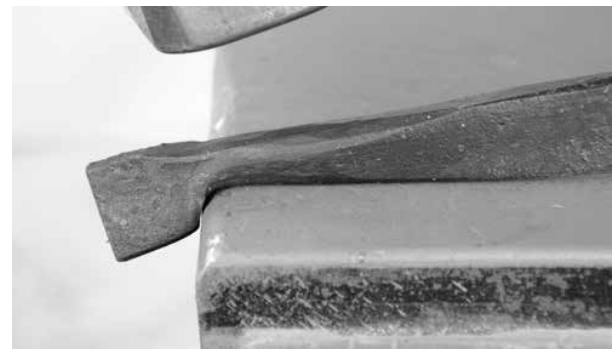
Finally take the neck to a round cross section without destroying the look of the taper to the parent bar
